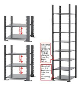
Step 4 Refer to the previous step. If the first support plate is not installed, install the other bracket in sequence.
