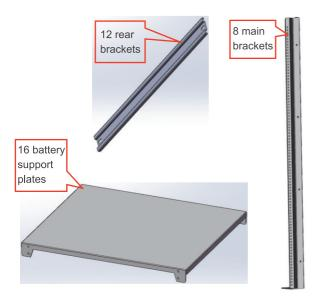
Step 2 As shown in the picture below, use M6\*16 screws to fix the support plate and main bracket.
